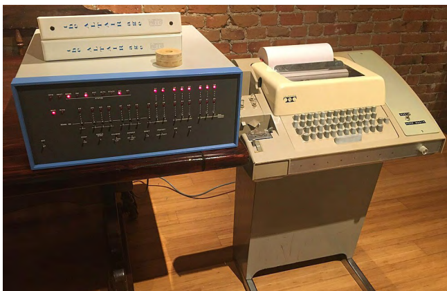
Altair 8800, the first commercially successful personal computers. Image: Wikipedia Commons - Tim Colegrove
